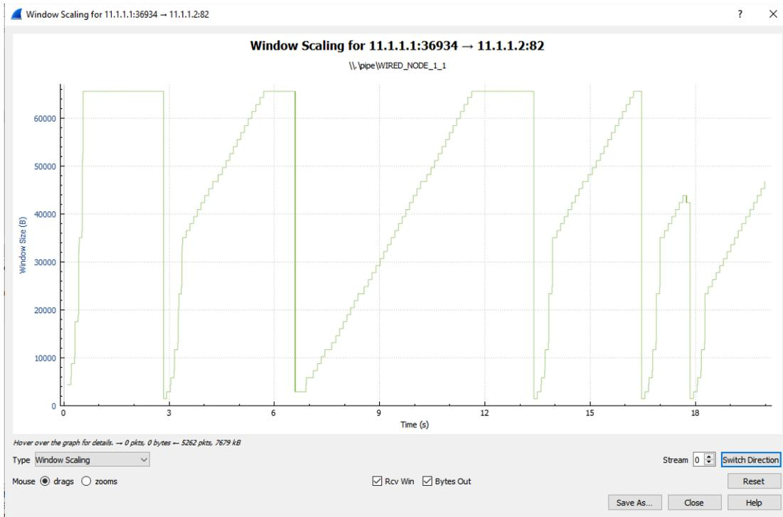
Figure 13-5: Congestion window evolution with TCP Tahoe. We note that Tahoe infers packet loss with timeout and triple duplicate acknowledgements, and updates the slow-start threshold  $ssthresh$  and congestion window  $cwnd$  as  $ssthresh = cwnd/2$  and  $cwnd = 1$
