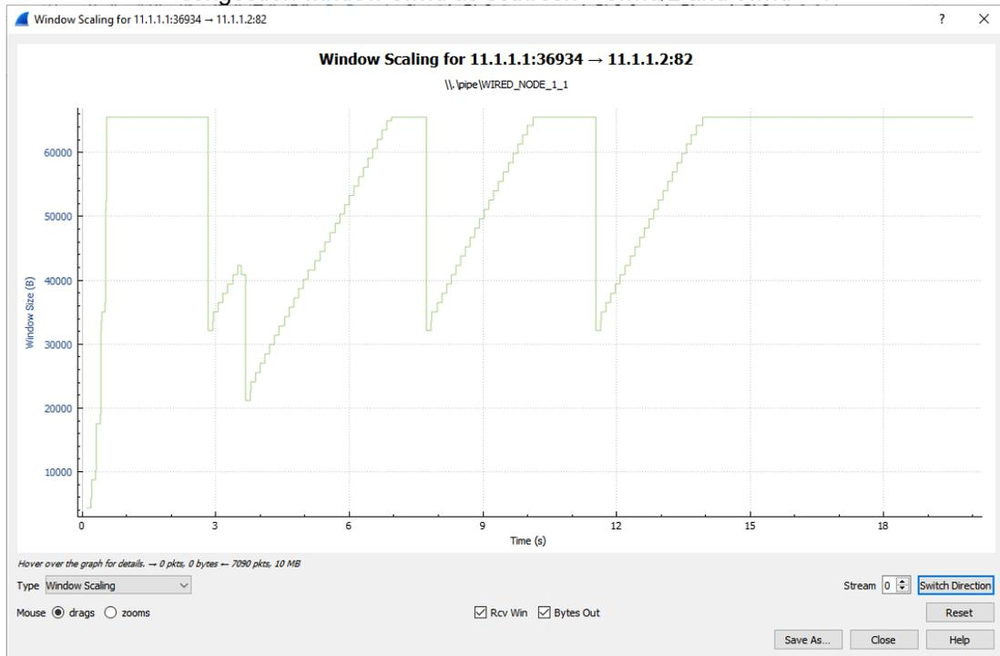
Figure 13-6: Congestion window evolution with TCP New Reno. We note that New Reno infers packet loss with timeout and triple duplicate acknowledgements, and updates the slow-start threshold  $ssthresh$  and congestion window  $cwnd$  as  $ssthresh = cwnd/2$  and  $cwnd = ssthresh + 3MSS$  (in the event of triple duplicate acknowledgements).
