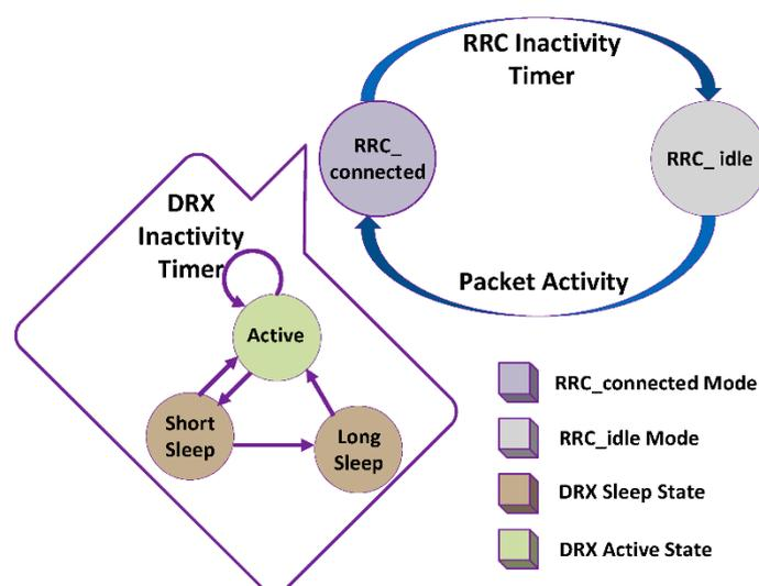
We design DRX as a three-state model as shown above. These states are (1) active state, (2) ON state, and (3) sleep state. The UE can receive packets during the active state. In case of no packet in the buffer, UE waits until the expiry of inactivity timer. If UE receives an intimation of packets arrival before
