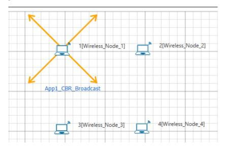
Wireless Node 1 initiates a broadcast message and the message is received by nodes 2, 3 and 4.2, 3 and 4 rebroadcast the message if they have not broadcasted that before. Furthermore, this implementation involves a Rebroadcast\_Probability based on which the nodes resend the packets.
