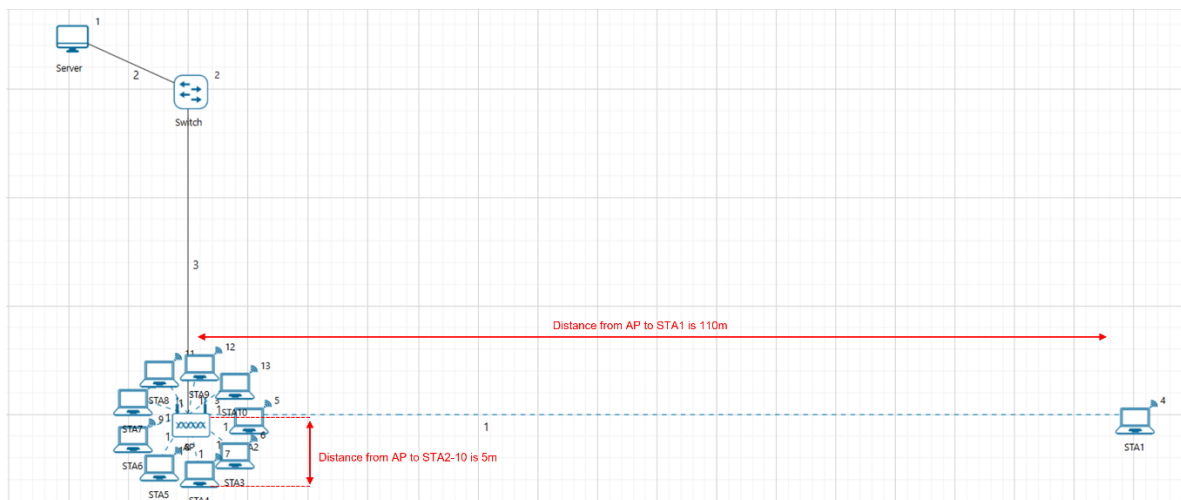
Figure 5: Network set up of 1AP-10STA scenario for studying the Impact of distance on Wi-Fi Throughput for 1 slow STA, Distance from AP to STA1 is 110m and MCS is 0 (slow STA), Distance from AP to other STA is 5m and MCS is 7. All STAs are generating saturation uplink traffic.
