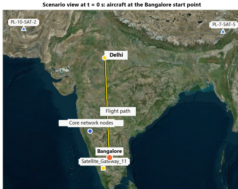
Figure 1-4: Scenario view at the start of the simulation, with the aircraft at the Bangalore start point at 0 s. The yellow line marks the configured flight path toward Delhi over the 0–7920 s simulation. The same view shows the core network nodes, the satellite gateway, and two of the visible satellites.
