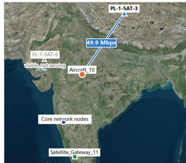
Figure 1-5: Two snapshots during the flight in the 100-satellite run. The blue link and the throughput badge identify the serving satellite at that instant. Early in the flight the aircraft is served by PL-1-SAT-1 at 28.5 Mbps; about an hour and a half later it is served by PL-1-SAT-3 at 49.9 Mbps, with other satellites visible but not serving. Serving-satellite intervals are taken from Table 1-3.
