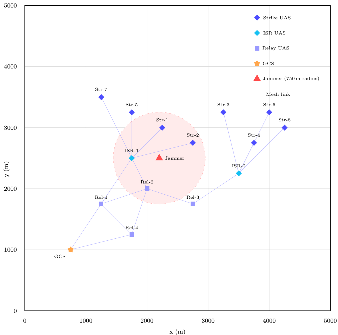
Figure 1: Network topology and initial node deployment. 8 Strike, 2 ISR, and 4 Relay drones form a multi-hop DTDMA mesh (L-band, AODV routing). Lines show primary mesh links. The shaded circle marks the jammer’s 750 m effective radius, which covers Strike-1, Strike-2, ISR-1, and Relay-2.
