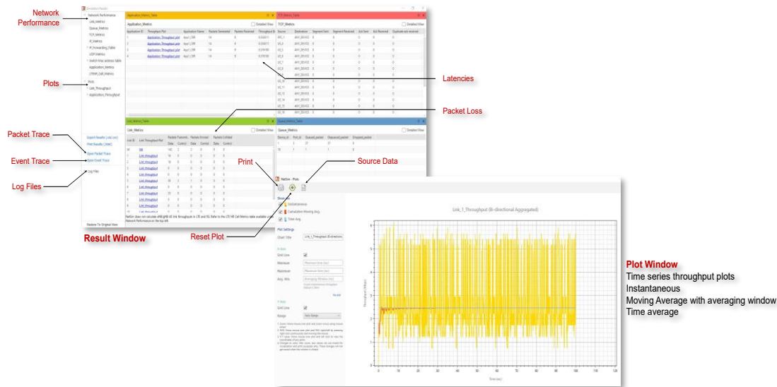
Figure 1-2: The Result dashboard and Plot window shown in NetSim after completion of simulation.
