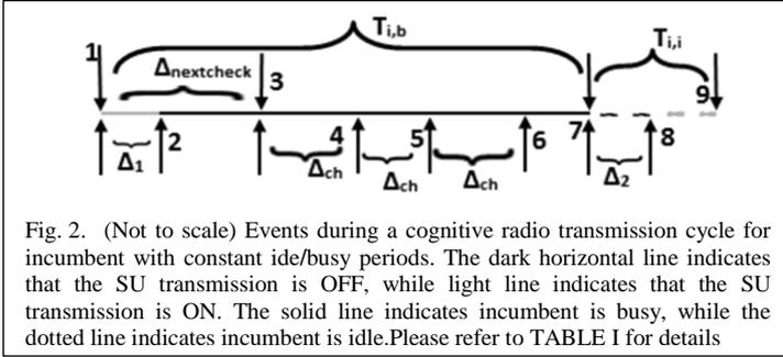
Fig. 2. (Not to scale) Events during a cognitive radio transmission cycle for incumbent with constant idle/busy periods. The dark horizontal line indicates that the SU transmission is OFF, while light line indicates that the SU transmission is ON. The solid line indicates incumbent is busy, while the dotted line indicates incumbent is idle. Please refer to TABLE I for details
