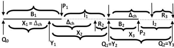
Fig 4. Events during a cognitive radio transmission cycle: for incumbent when idle and busy time of the incumbent follow exponential distribution. Different cycles are labelled as  $X_i$ .  $B_i$  and  $I_i$  are the durations of the  $i^{th}$  busy and idle periods respectively.  $R_i$  represents the reward in the  $i^{th}$  cycle.  $X_1$  belongs to case 1 (so  $R_1 = 0$ ), while  $X_2$  and  $X_3$  belong to case 2 (they have nonzero rewards).
