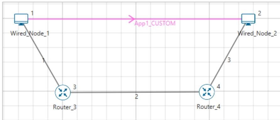
Figure 1-6: Network set up for studying a single flow
