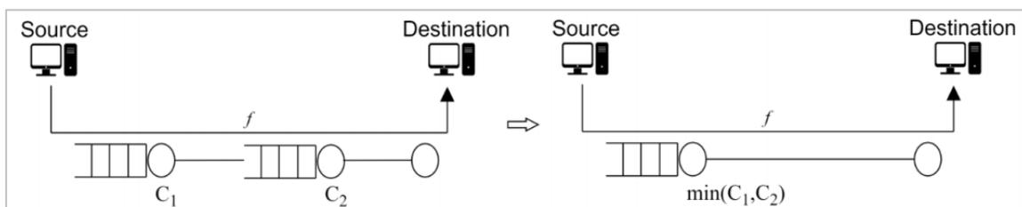
Figure 1-3: Approximation of a network using bottleneck server technique
