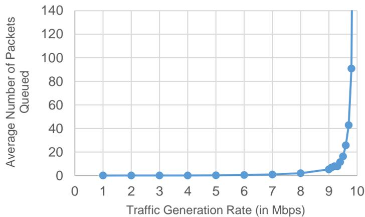
Figure 1-20: Average queue (in packets) at the bottleneck link 2 (at Router 3) as a function of the traffic generation rate
