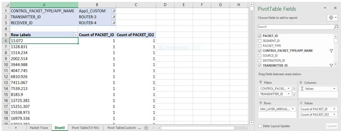
Figure 1-15: Adding fields into Filter, Columns, Rows and Values
