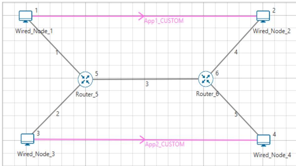
Figure 1-21: Network set up for studying two flows
