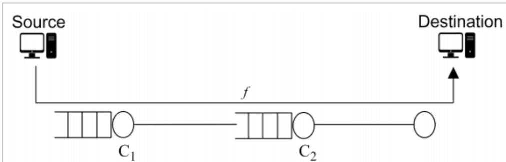
Figure 1-2: A single flow  $f$  passing through a series of links. The link with the least capacity will be identified as the bottleneck link for the flow  $f$
