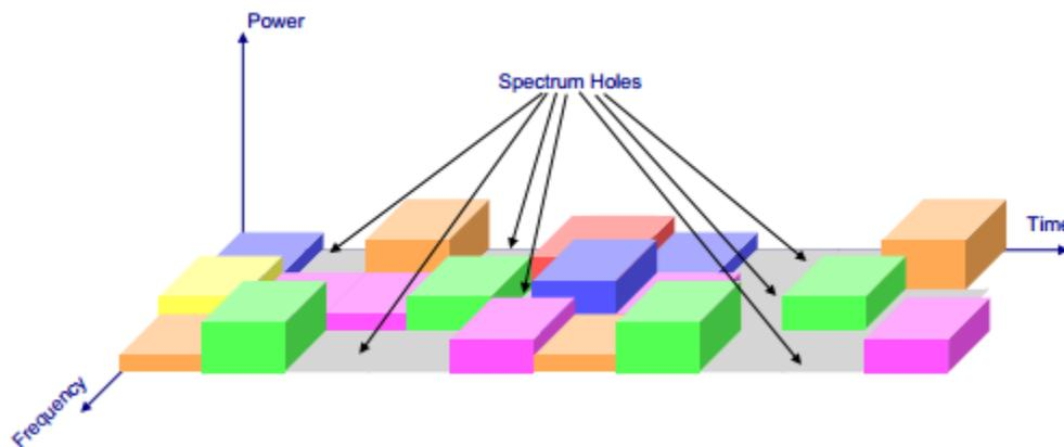
Figure 1-1: Spectrum holes are used by SU for its transmission scheme is often referred to as opportunistic spectrum access (OSA)
