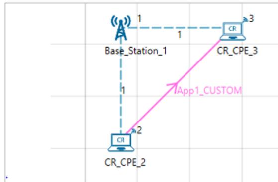
Figure 1-4: Network set up for studying the Frequency allocation to PU and SU
