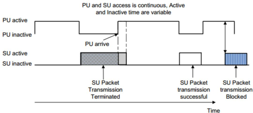
Figure 1-2: Illustration of forced termination and blocking of a SU connection
