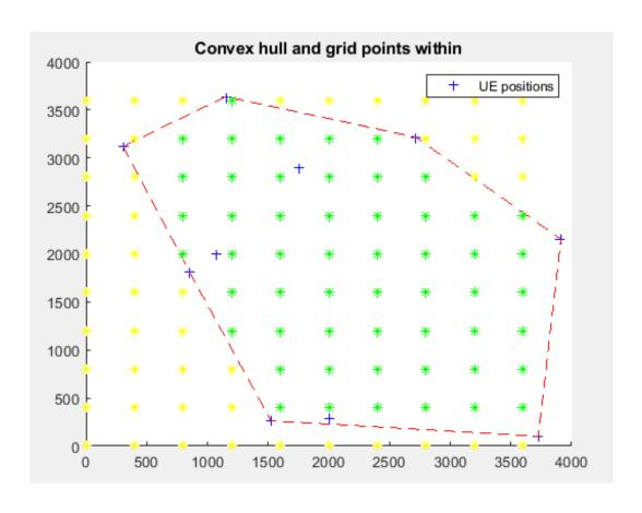
The green markers are the points where the base station can be placed. At each point the sum throughput is computed. We then pick the point with maximum aggregate throughput
